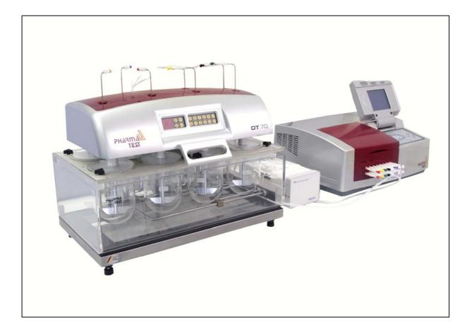
Simultaneous stirrer start, manual or automated operation is offered by the advanced ADS DT70 System. It includes a Ismatec Multi Channel Peristaltic Pump and a Pharma Test T70 UV/VIS Spit-Beam Spectrophotometer or a any other suitable UV/VIS Photometer with 8-cell changer. The fully automated closed loop Tablet Dissolution Testing System is controlled by the WinDiss32 Software Suite which is fully 21CFR Part 11 compliant.
